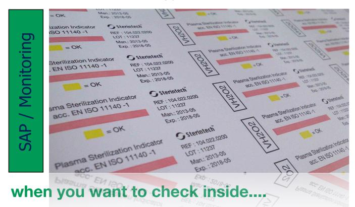
These indicator strips can be used as in-pack indicator in order to detect sterilization conditions have been met inside the pack.
